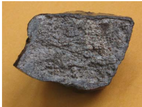
Figure 6.- Free face after cutting. Surface coating is artificial resin not a reaction crust. Fragments in all photos are 4-5 cm. tall.
